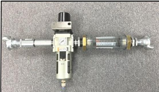
Compressor Air Pressure Reducer and Air Flow Regulator
