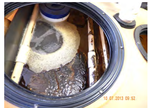
Iron Bacteria Separated from Fuel by DAF and \text{CaCl}_2 Flocculation
