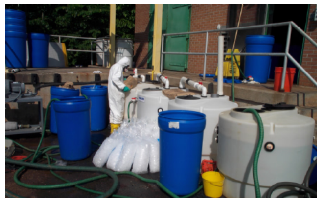
Burn Residue Dechlorination Reactors
