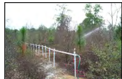
HC2 Gasoline Wetland 5 Month Biostimulation System
