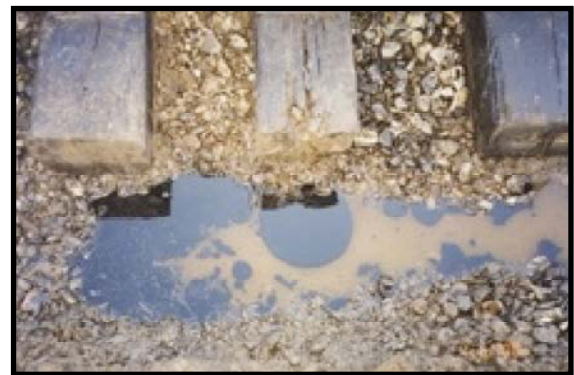
Desorption of Lube Oil from Ballast with HC-2000
