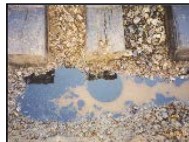
HC-2000 Desorbs & Degrades Lube Oil in Railroad Ballast
