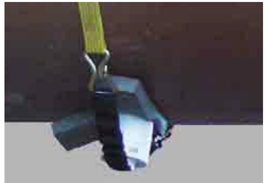
Bottom Outlet Valve Can Cover
