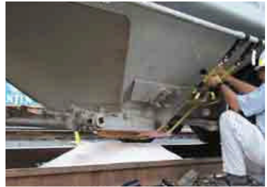
Leaking Sodium Phosphate Hopper Car Patched
