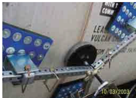
Gasket Compression Against Container over Weld Seam
